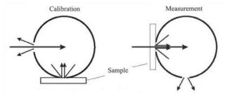
4). Open measurement area, no limit on sample size.
